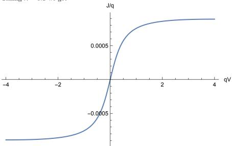
Note that the current saturates when all the left-moving states are filled, and all of the right-moving states are empty.
